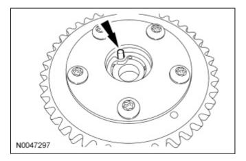
3. Visually inspect the camshaft phaser and sprocket for squareness (A). If the trigger wheel or spring is deformed or damaged (B), install a new camshaft phaser and sprocket.
